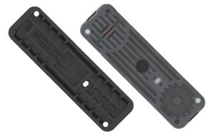
ND emitters eliminate drainage and refill effect, and improve efficiency in pulse irrigation. In order to achieve the Non-Drain function, the emitter closes when the pressure is below 0,1 bar.
